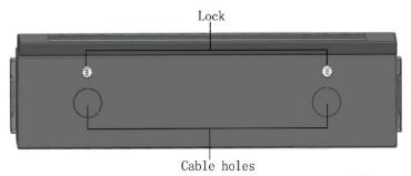
1. Remove one of the bottom covers to pass cables for TV and fan through. Insert rubber gasket into hole.
