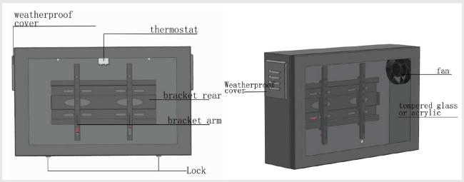
**PART** A: Enclosure \* ..... B: Tempered Glass\* ..... D: Fan \* ..... E: Thermostat\*.... G: Hardware (at right) .....1 H: Key ......2 1: Rubber Gaskets.....2 J: Rod\*.....2 Expansion screw \*: Arrives assembled NOTE: 2-3 person assembly Tools Required: Drill; Phillips
